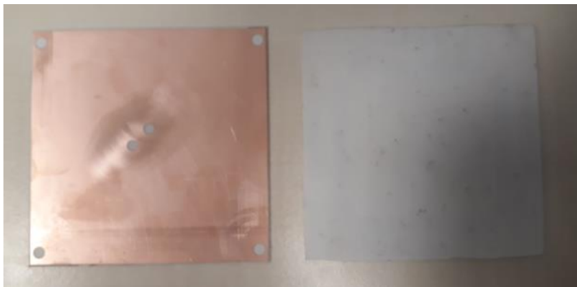
Figure 3.15 Bottom sides of the active and parasitic layers of the fabricated antenna
